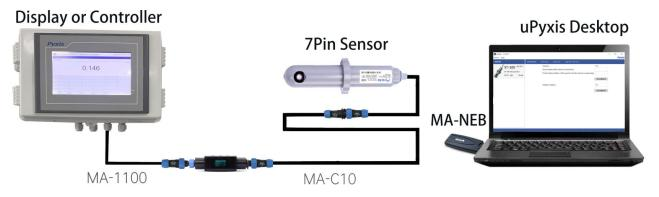
Figure 13. 7-Pin Sensor with MA-WB and MA-NEB and uPyxis Desktop
