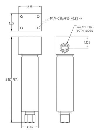
Figure 4. Dimension of the ST-500SS (inch)
