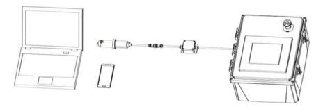
Figure 4. Bluetooth connection to ST-525 Series sensor
