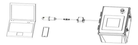
Figure 4. Bluetooth connection to ST-588 sensor
