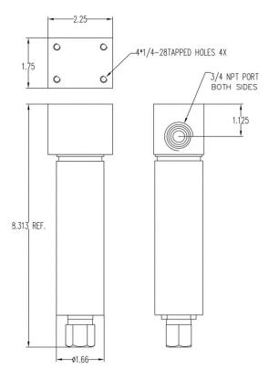
Figure 3. Dimension of the ST-588SS (inch)
