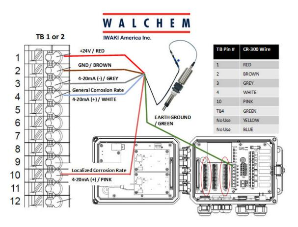
Figure 10. Typical wiring for WalChem W600
