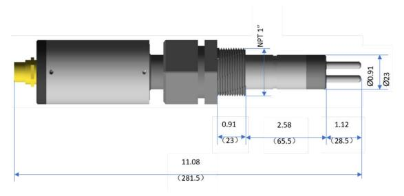
Figure 4. CR-300 Series Dimensions in inch (mm)
