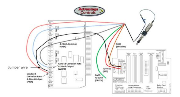
Figure 14. Typical wiring for Advantage Controls MegaTronXS
