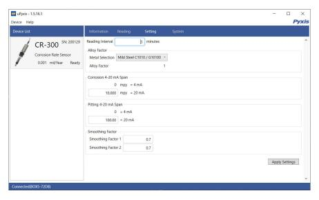
Figure 30. Select metal type, 4–20 mA output scale, and reading interval
