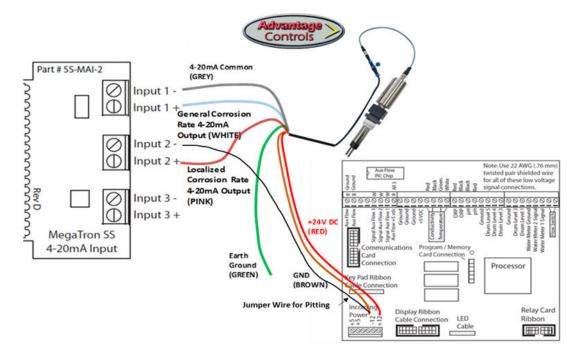
Figure 13. Typical wiring for Advantage Controls MegaTron SS
