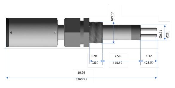
Figure 3. CR-200 Series Dimensions in inch (mm)
