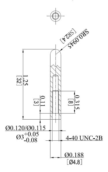
Figure 16. Test Metal Electrode Dimensions, Inch [mm]
