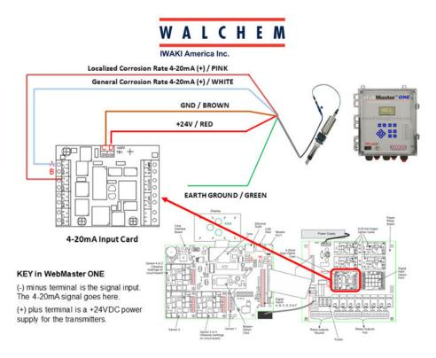
Figure 12. Typical wiring for WalChem WebMaster One
