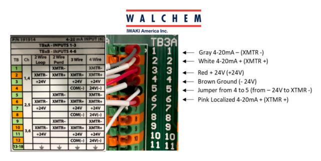
Figure 11. Typical wiring for WalChem W900 (4-wire loop configuration)
