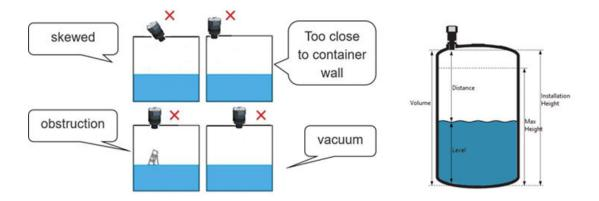
Figure 3. Installation illustration
