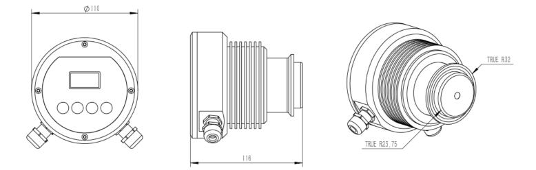
Flow Assembly Dimensions (mm)
