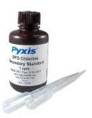
Figure 29. DPD Chlorine Secondary Standard 1 ppm
