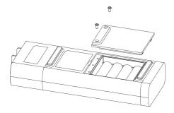
Figure 1. The SP-710 battery compartment
