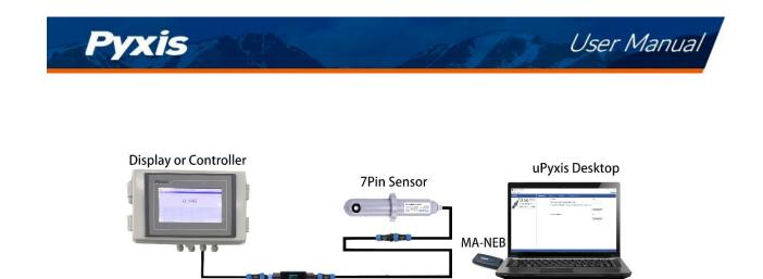
Figure 11. Bluetooth connection to ST-601 sensor with MA-WB and MA-NEB and uPyxis Desktop App.
