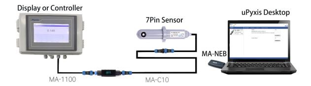
Figure 12. USB connection to ST-730 Series sensor with MA-WB, MA-NEB and uPyxis Desktop App.
