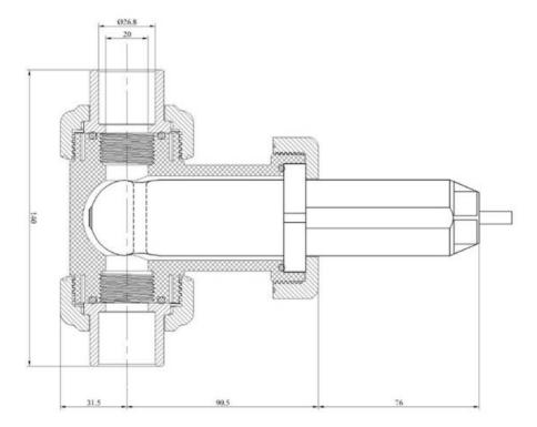
Figure 3. Dimension of the ST-730/730B/731/735 and the ST-001 Tee Assembly (mm)
