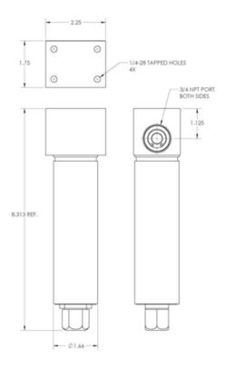
Figure 4. Dimension of the ST-730SS (inch)
