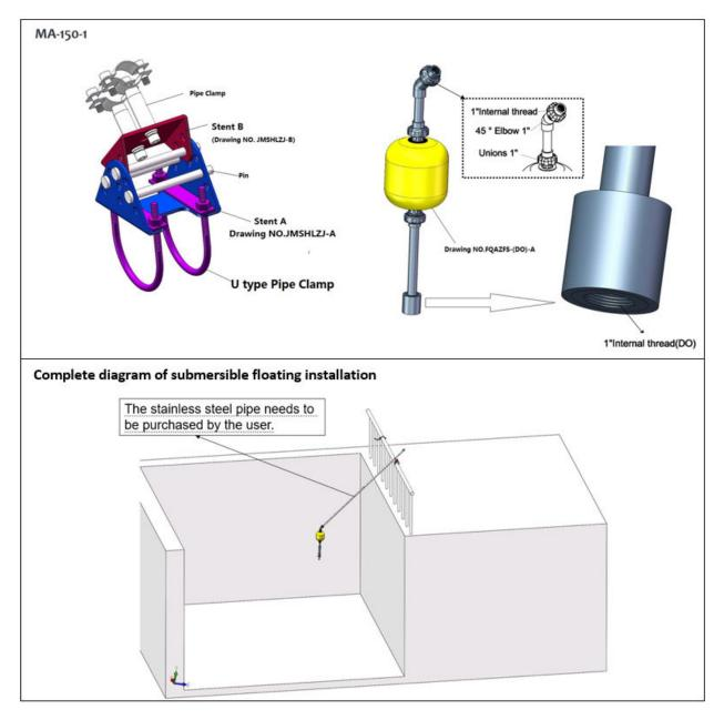
Figure 1. ST-772/ST-772-P in a submersed floating installation
