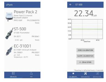
7. Press on the image of desired sensor. uPyxis will default to Calibration page. User can view sensor readings, real-time trend chart and calibrate the sensor.
