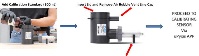
\*NOTE\* Sensor Brace Included with L-CAL Kit for Stability
