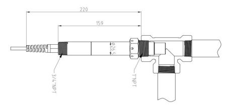
Figure 4 - ST-773 in the 1-inch Threaded Adapter Kit (P/N 50700-A04)
