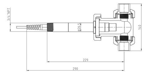
Figure 5 - ST-773 installed in the ST-001 Tee + Collar Assebmly Kit (P/N 53726)
