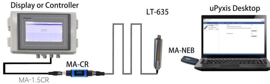
Figure 17 - Connect the LT-635 to a computer via Pyxis MA-CR and MA-NEB adapter
