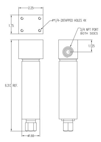
Figure 3. Dimension of the ST-525SS (inch)
