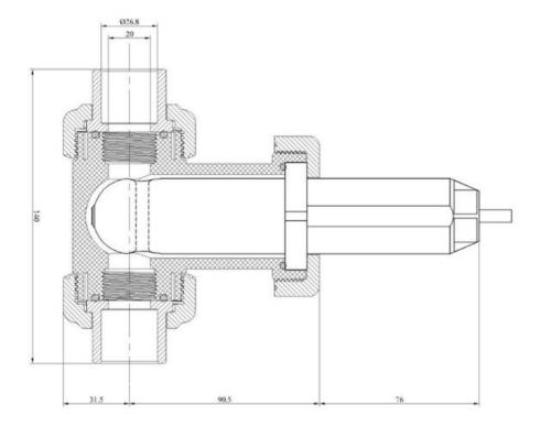
Figure 2. Dimension of the ST-525 and the ST-001 Tee Assembly (mm)
