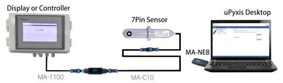
Figure 4. Bluetooth connection to ST-525 Series sensor
