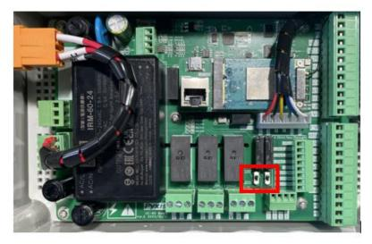
Figure. 19 – Relay Active/Passive Toggle Switch on UC-80 Terminal Board
