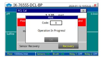
Figure. 44 – In Progress Screen of Free Chlorine Calibration
