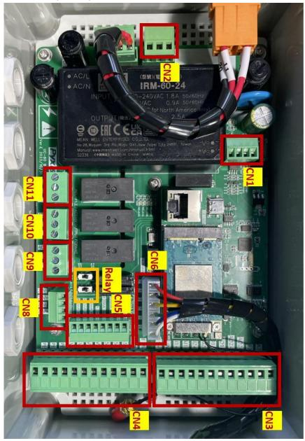
Figure. 3 – Terminal board of the UC-80 Display
