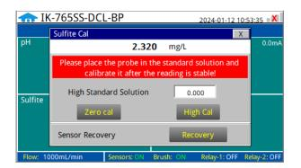
Figure. 45 - Sulfite Calibration
