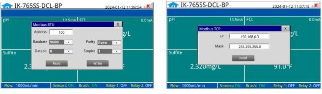
Figure. 37 - Modbus RTU
