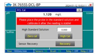
Figure. 43 – Free Chlorine Calibration of ST-765SS-FCL
