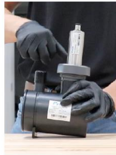
Tighten Sensor Nut
